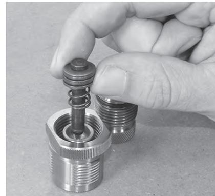
③ Re-install adjustment knob several turns to engage the coil spring.
