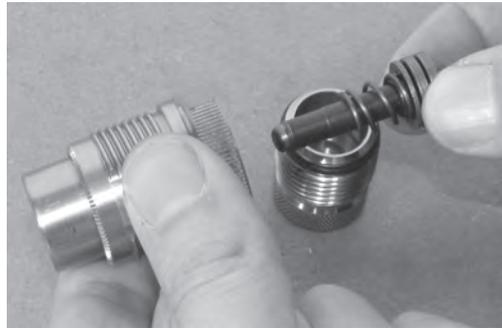
② Install coil spring into compression plug followed by the correct swage punch assembly (small or large).
