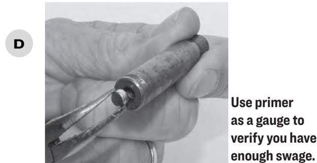
Be sure you push hard enough on the lever to reach the press stop to assure consistent swages. Properly adjusted, it takes approximately 30 pounds on the lever to swage large primer size pockets. If you can't reach the press stops with 30 pounds of pressure on the lever, you have the swage punch set too deeply.
